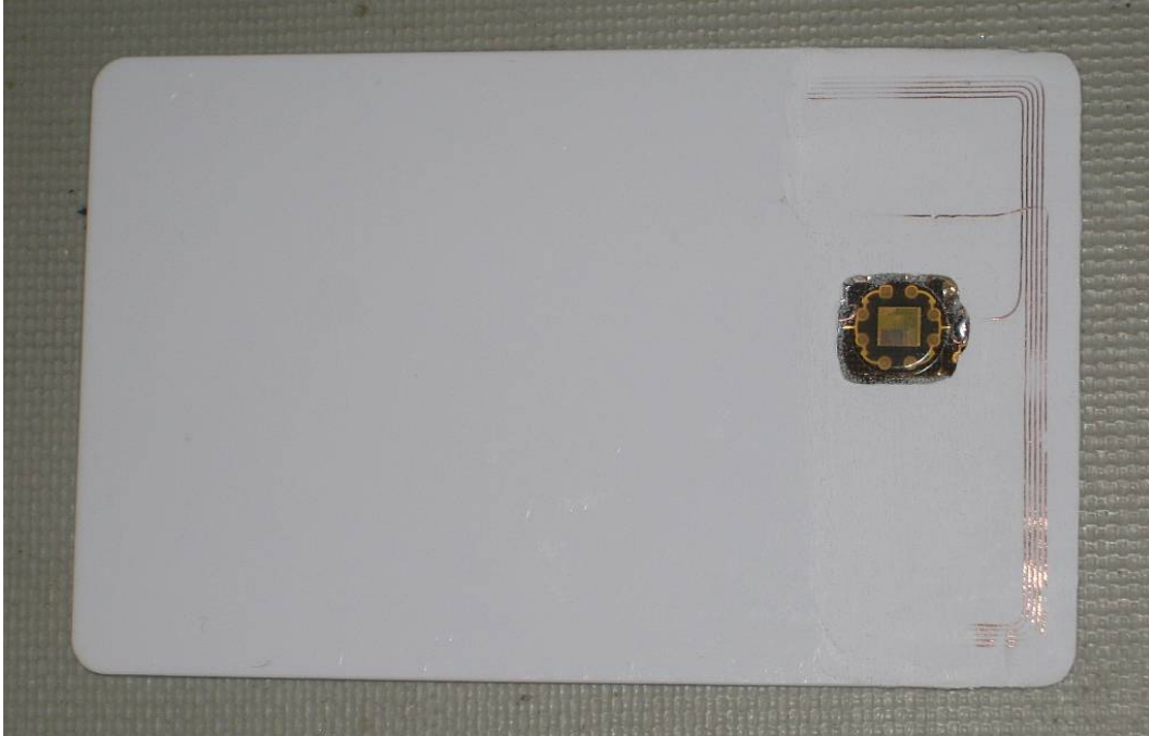
Figure 2.6: Antenna Beneath Contactless Card Surface
